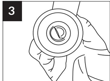
**PUSH** the valve onto the bottom of the flange.
