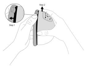
2. Remove the diaphragm from the groove.
