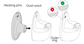
3. Press firmly behind the heating pins for full extension. Heating may fail if not fully extended.
