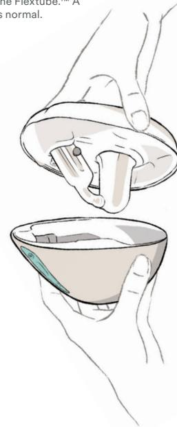
fig 4l If more than a few drops are present, turn Pump back on, attach Flange, Press Pump/Pause button and repeat Flip to Finish.
