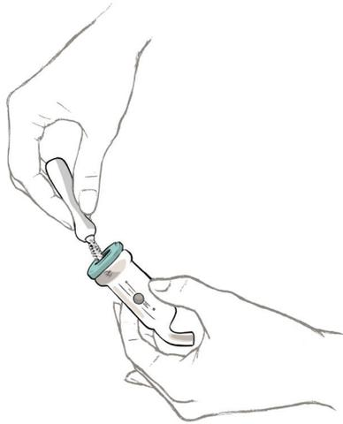
fig 5d Insert small brush into Tip at bottom and clean.
