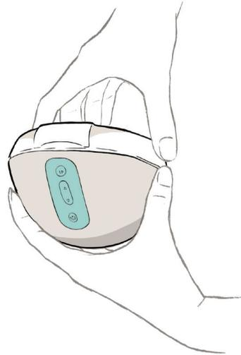
TIP: To easily separate Flange from Pump, hold near the bottom and pull apart.
