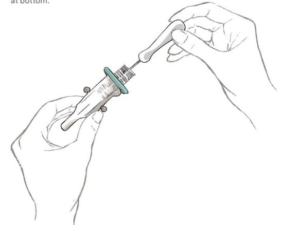
fig 5c Use small brush to clean inside top opening and area under Collar.
