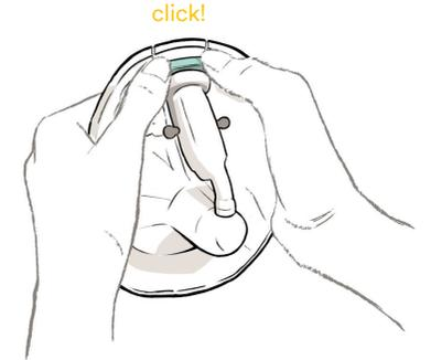
TIP: Flextube™ must be pushed all the way down onto the Flange Spout.
